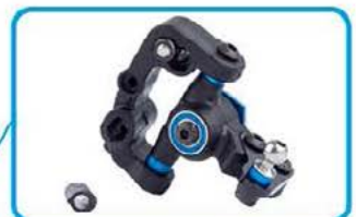
One-piece steering blocks with bolt-on Ackermann plate
