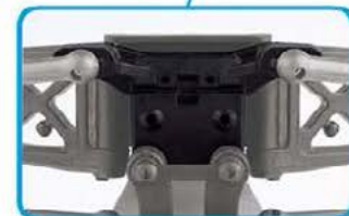
Front and rear sway bar integration makes tuning easy (sway bars not included)
