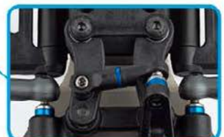
Reverse bell-crank steering rack design allows more room for electronics
