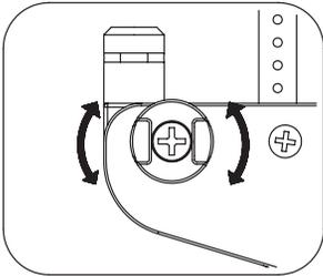
**Note:** Upper Shock mounting should be able to turn 360°. Do not overtighten the screw.
