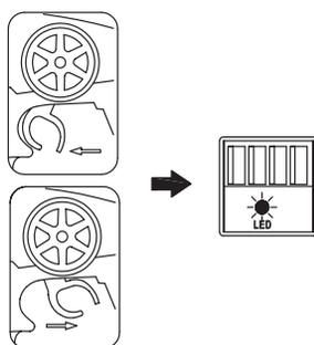
The LED of the ESC will be switched on during forward and backward mode. LED will only turn off, when switch is set to „off“-position, or no battery is connect.
