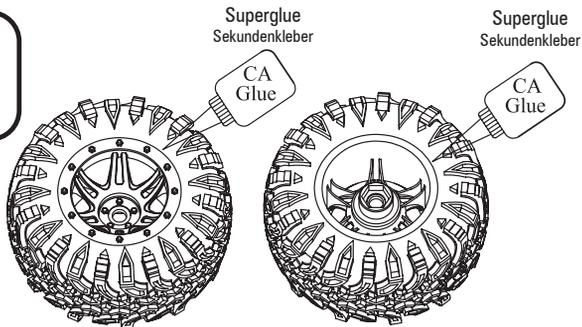
Use Superglue to attach the tires to the rim. Lift the tire, to let the superglue flow between the tire and the rim.
