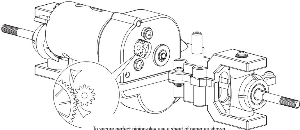
To secure perfect pinion-play use a sheet of paper as shown
