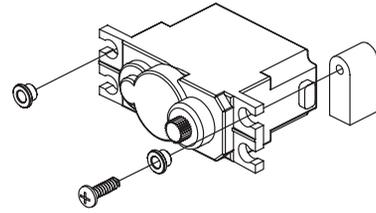
**Note:** If installing Acorns or JR-Servos, please use the two washer as shown above
