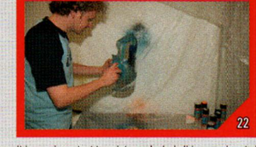
It is very important to paint your bodyshell in a good vented room at 20°C to 25°C environmental temperature.
