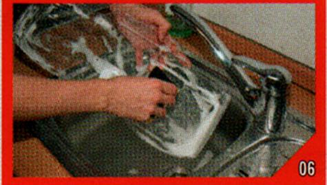
Clean the bodyshell with water and dish washing liquid and let it dry - best overnight. Don't blow-dry it, because that would bring up dust to the body shell again!
