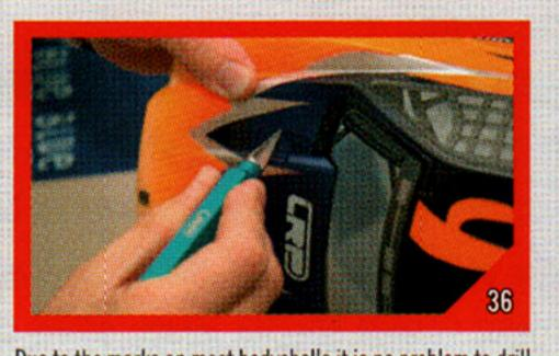
Due to the marks on most bodyshells it is no problem to drill correct mounting holes. The easiest way is to drill the holes with the LRP Body Reamer (#65701).
