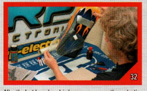
After the last layer has dried, you can remove the protective film from the outside.
