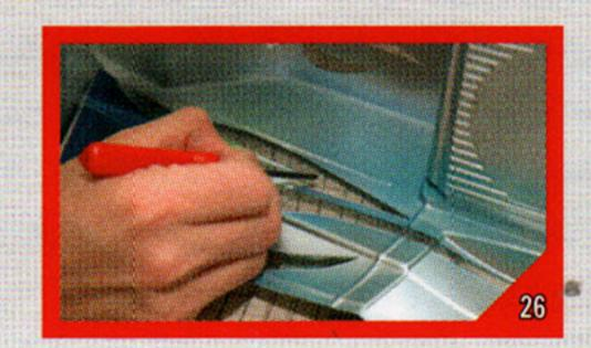
Here some colour ran under the masks. Sasha removes it carefully with a knife.
