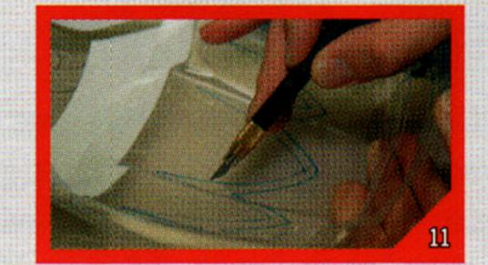
Cut the masks very carefully along the lines. Do not damage the bodyshell! You can try with the left-over cuts from the fenders before.
