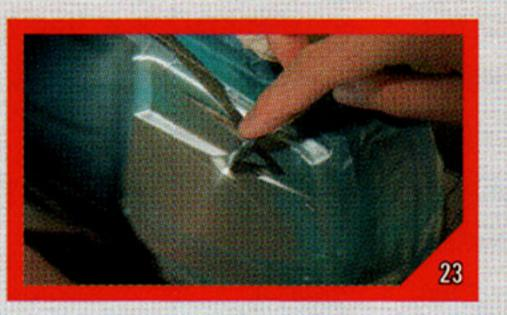
While the colour is still wet, carefully remove the masks for the chrome area.
