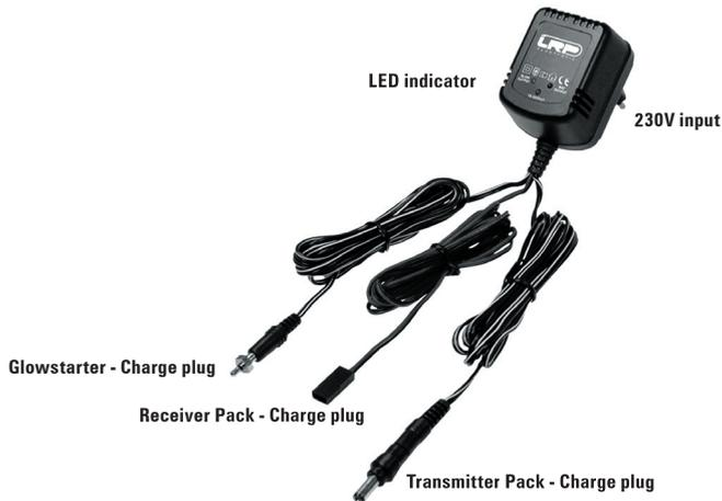
The 3in1 charger has been specially developed to simultaneously charge 3 batteries at once. You can charge Transmitter packs (TX), Receiver packs (Bat) and Glow Starter batteries (Glow) either simultaneously or individually. You can also charge a 6 cell SubC battery pack over the Transmitter output (TX) using a special charging adapter. The charger has to be plugged into a standard 230V power socket and is ready for use straight away.
