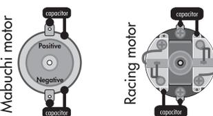
**ONLY FOR BRUSHED MOTORS!** Motors with no capacitors or not enough capacitors may interfere with the speed-control. To avoid this, solder the supplied capacitors to your motor (see picture).
