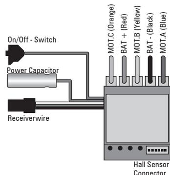
**RECEIVER CONNECTING WIRE:** The *Ultimo Drift* is equipped with an LRP Multicon receiver wire. As supplied, it will easily fit in all ordinary receivers. Make sure you connect it to receiver with correct polarity and use channel 2.
